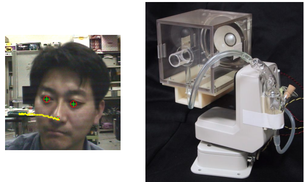
Figure 1. System components: a vision-based nose tracker and a scent projector using an “air cannon.”
