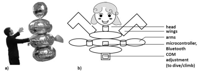
Fig. 2. A prototype flying humanoid robot (FHR), Angel: a) interacting with a person, b) system architecture
