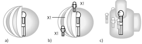
**Fig. 3. 3D positioning space for a robot: a) simple sphere model (stripes represent F-formation equilibria), b) problems with the simple model (a FHR can be too close to head or feet and face should be seen) c) proposed model for 3D with equilibria**
