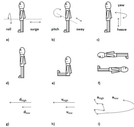
**Fig. 5. Kinesics of flight for a humanoid robot: a-c) primitive motions, d-f) postures (standing, sitting, lying) g-i) style of flight: high/low displacement, velocity, acceleration (insect-like or bird-like)**
