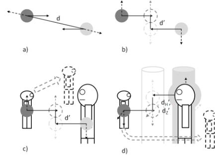
**Fig. 4. Modeling 3D collision avoidance with social forces: a) difficult case for Spherical Specification (SpS), b) a solution via Collision Prediction (3CP) c) difficulty of using spherical fields for humans in 3D, d) proposed model**
