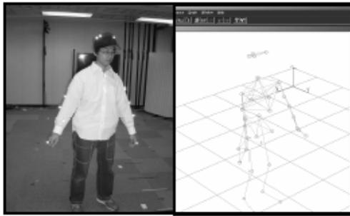
Fig. 7: Vicon motion-capturing system
