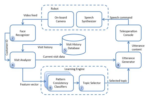
Figure 4. Architecture of the greeting system used in the field trial. Numbered elements correspond to elements presented in Fig. 1. Elements 1, 3, and 9 are not present here because the tracking system, sensor fusion, and training interface were not used in the field trial
