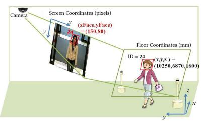
Figure 3. Illustration of sensor fusion between a camera and the position tracking system. The positions of people in the floor coordinate system detected by the position tracker are projected into the screen coordinates of the camera system. Nearest-neighbor matching is then used to associate face ID's with anonymous pedestrians detected by the tracking system
