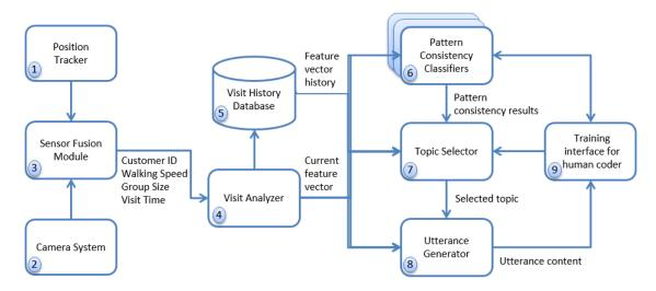
Figure 1. Data flow for training phase. System elements are numbered for reference in the text. Sensor data is used to generate feature vectors which are used as inputs to pattern consistency classifiers and topic selector. A human coder provides training data for the classifiers
