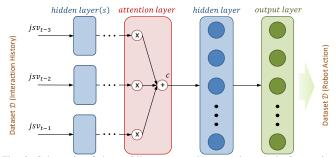
Fig. 2. Schematic of the multilayer perception neural network. Interaction history is inputted to the neural network as joint state vectors and robot action as training target for the neural network.
