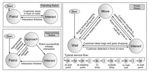
Figure 18. State transitions for service tasks in our field trial.
