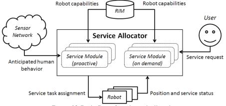
Figure 13. Basic flow of service task allocation
