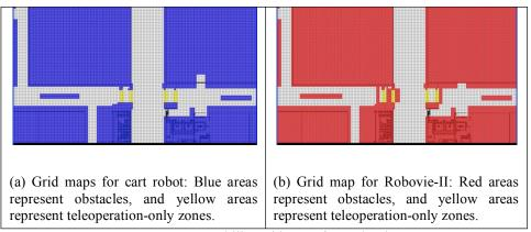
Figure 11. Traversability grid maps for each robot type.
