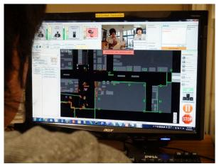
Figure 15. Operator using a teleoperation console to supervise four robots.
