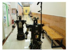
Figure 8. Deadlocked robots unable to pass each other in a corridor.
